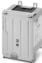
Battery module (device with battery), Lithium-Ion (LiFePO<sub>4</sub>), 24 V DC, 128 Wh. For use with a QUINT UPS for ambient temperatures (charging) of 0°C ... 60°C and a maximum charging current of 5 A. For charging below 0°C, please note the permissible UPS V/C level. 2 x 1446073 are required as replacement batteries.
