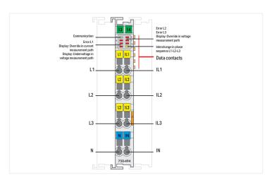
The 750-494 3-Phase Power Measurement Module measures electrical data in a three-phase supply network.
