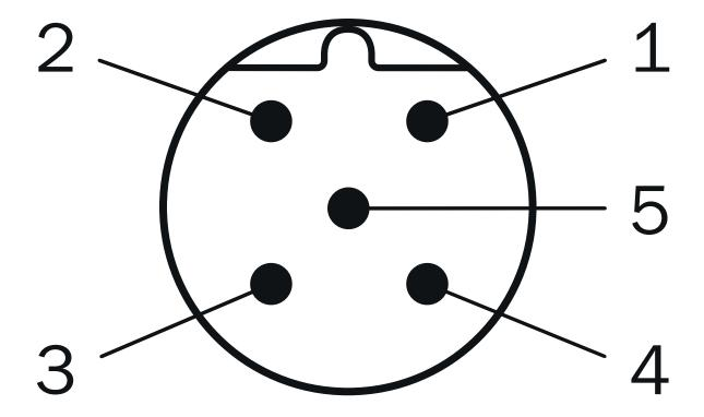
Connector M12, 5-pin, A-coded
