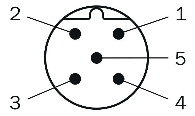
Connector M12, 5-pin, A-coded
