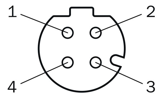
M12 female connector, 4-pin, D-coded
