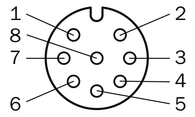
female connector M12, 8-pin, A-coded
