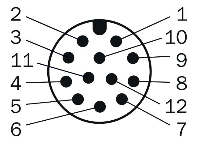
M12, 12-pin male connector, A-coded
