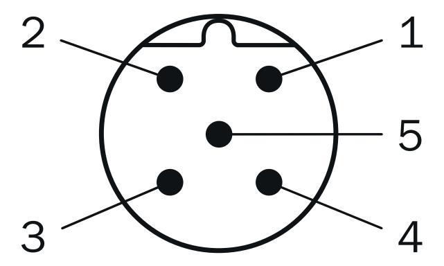
male connector M12, 5-pin, A-coded
