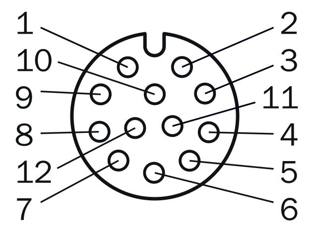
M12, 12-pin female connector, A-coded
