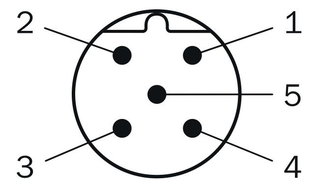
male connector M12, 5-pin, A-coded
