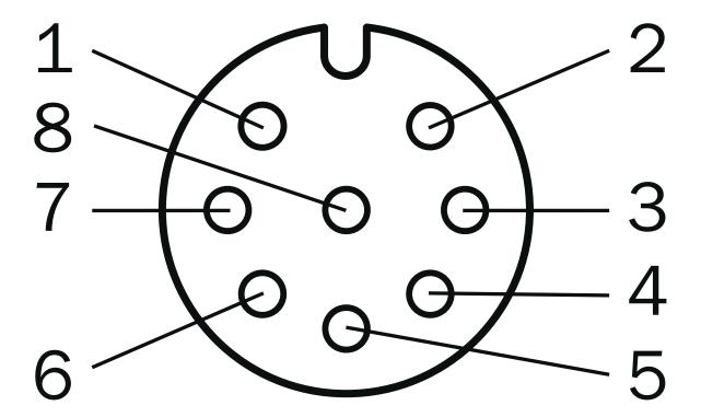
female connector M12, 8-pin, A-coded
