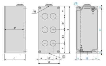
1 hole, with blanking plug (protrusion 6 mm/0.24 in.), for cable gland ISO M20 x 1.5 1 hole, without blanking plug, for cable gland ISO M20 x 1.5 2 x  $\varnothing$  5.6 mm/0.22 in. holes, depth 19 mm/0.75 in. (1) : (2) : (3) : P :
