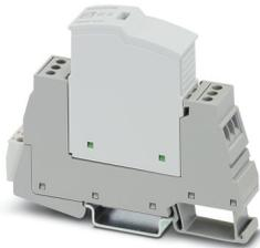
Type 3 surge protection, consisting of protective plug and base element, with integrated status indicator and remote signaling for single-phase power supply networks. Nominal voltage: 24 V AC/DC
