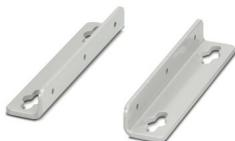
2-piece universal wall adapter for securely mounting the device in the event of strong vibrations. The profiles that are screwed onto the side of the device are screwed directly onto the mounting surface. The universal wall adapter is attached on the left/right.
