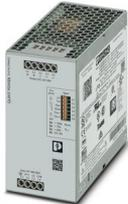
Preconfigured and read-only version of the primary-switched QUINT POWER power supply with set output voltage and adjusted signaling, input: 3-phase, output: 24 V DC / 20 A
